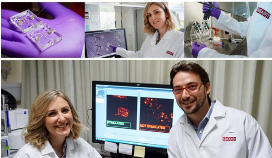
(L to R): PDMS microfluidic device with embedded electrodes; Lung cancer aggregates in the 3D hydrogel within device, in co-culture with non-cancerous cells; Injecting lung cancer cells into device
