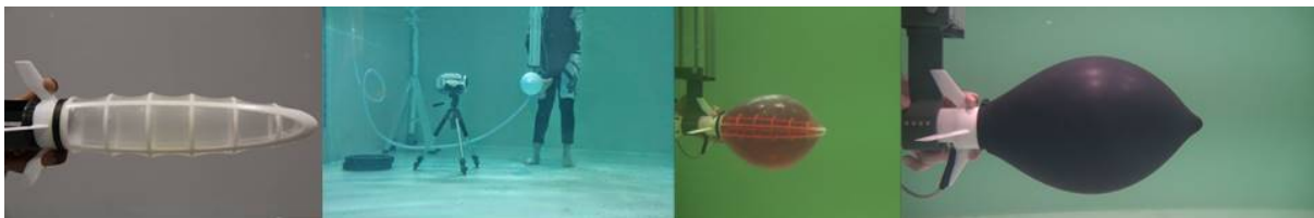
Fig.1: (L -R): Polycarbonate skeleton of robot, testing apparatus, fully blown membrane (last two pix)
