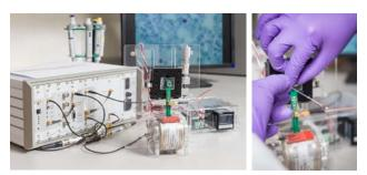
(Left) SMART developed the low-cost benchtop Magnetic Resonance Relaxometry system for rapid label-free malaria screening. (Right) Only a drop of blood is blood required for testing.
